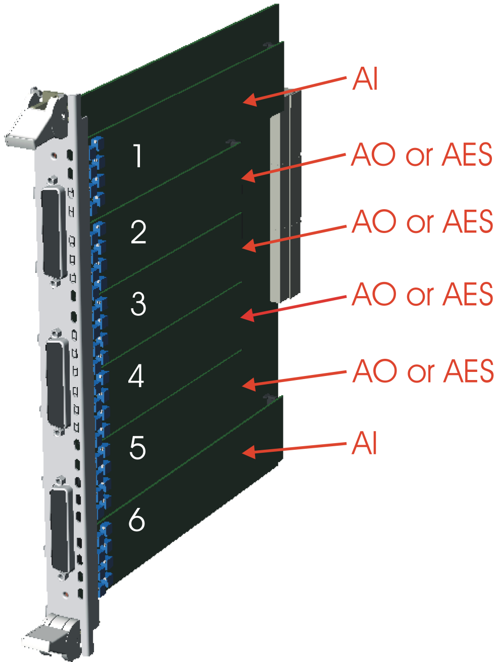
QDC Card with 6 Mezzanine Cards Connected
